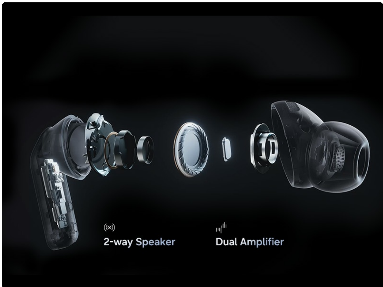
Image: An exploded view of a Galaxy Buds4 Pro earbud, illustrating its internal 2-way speaker and audio system.
