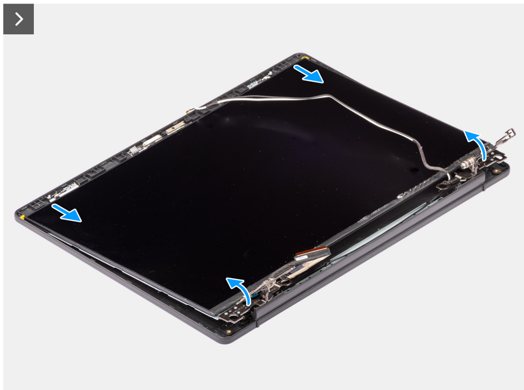
Figure 76. Removing the display panel
