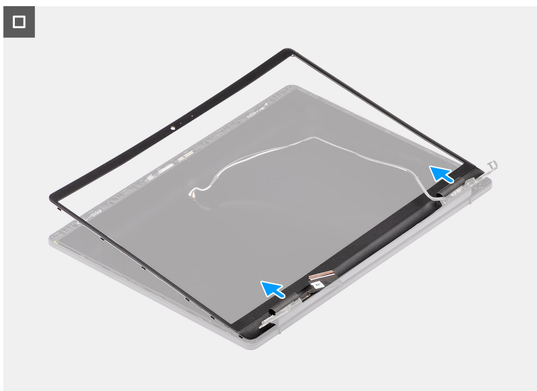
Figure 70. Removing the display bezel
