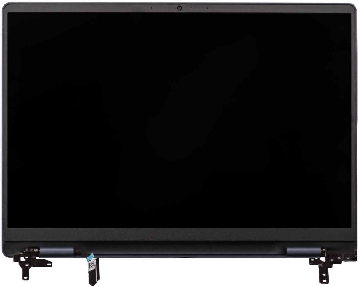
Figure 65. Display assembly (for computers shipped with an aluminum chassis)
