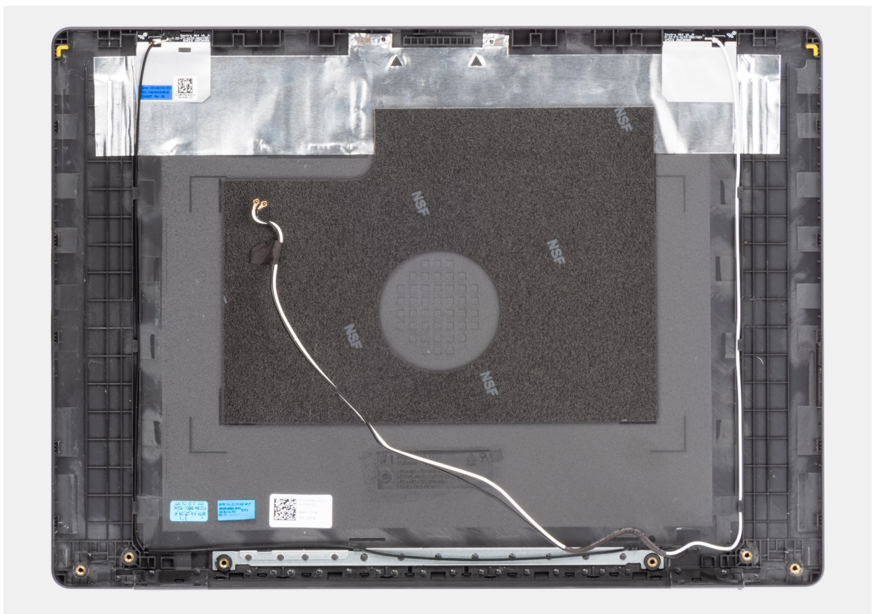
Figure 87. Display back-cover and antenna assembly
