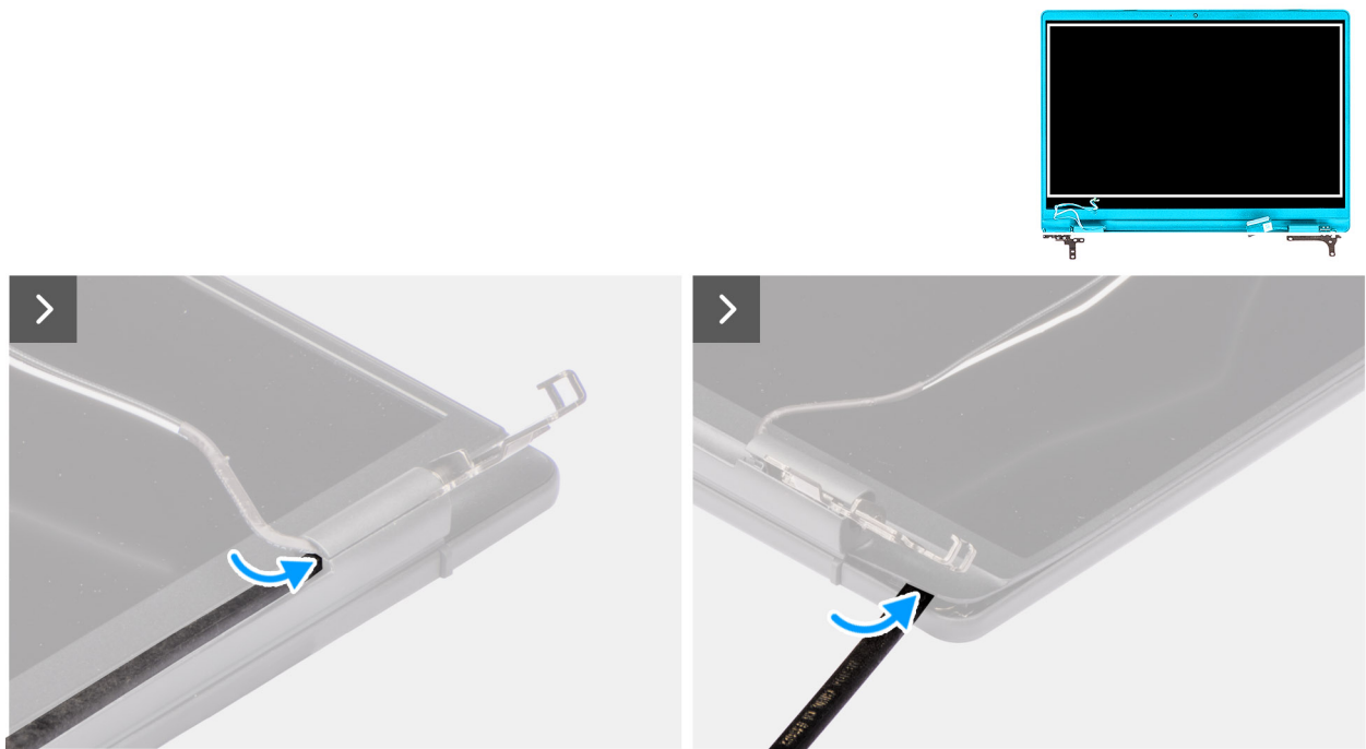
Figure 68. Removing the display bezel
