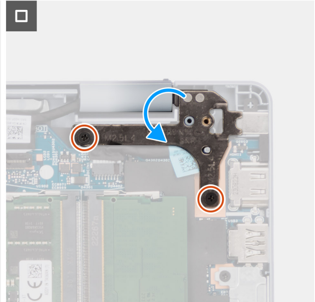
Figure 52. Installing the power-adaptor port (for computers shipped with a plastic chassis)
