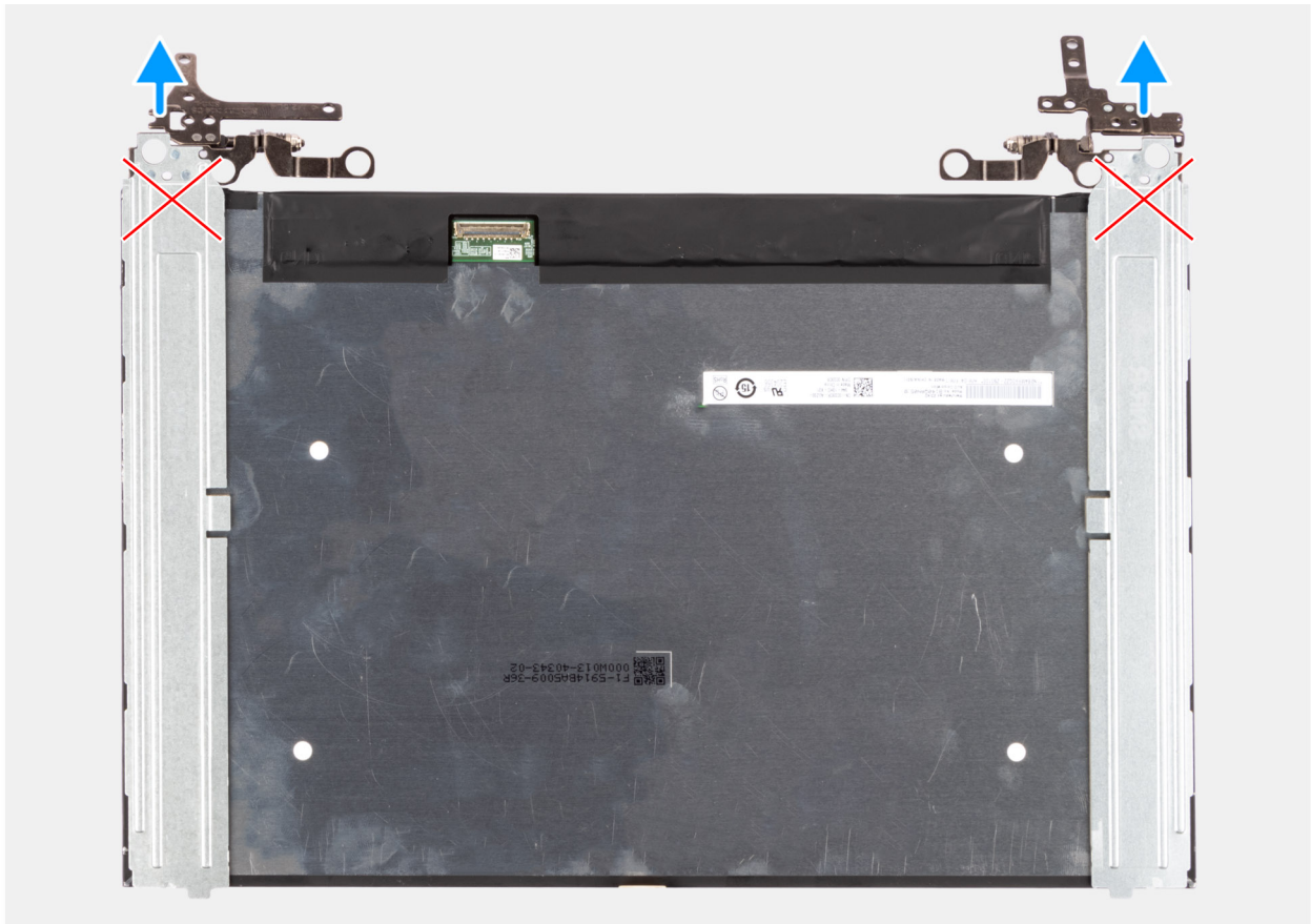
Figure 78. Removing the display panel
