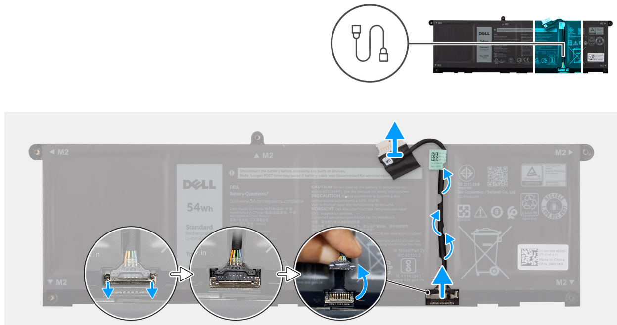
Figure 36. Disconnecting the battery cable
