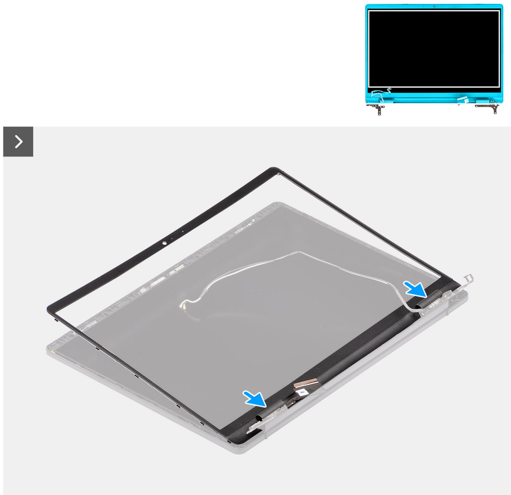
Figure 72. Installing the display bezel
