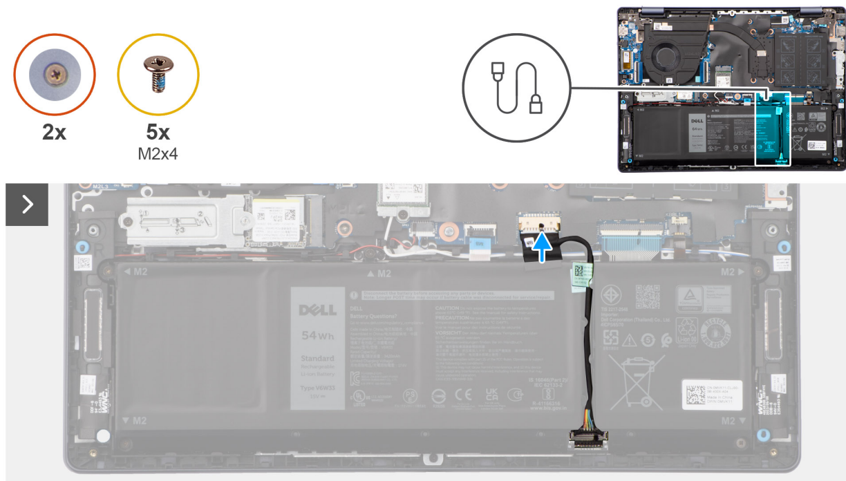
Figure 21. Connecting the battery cable
