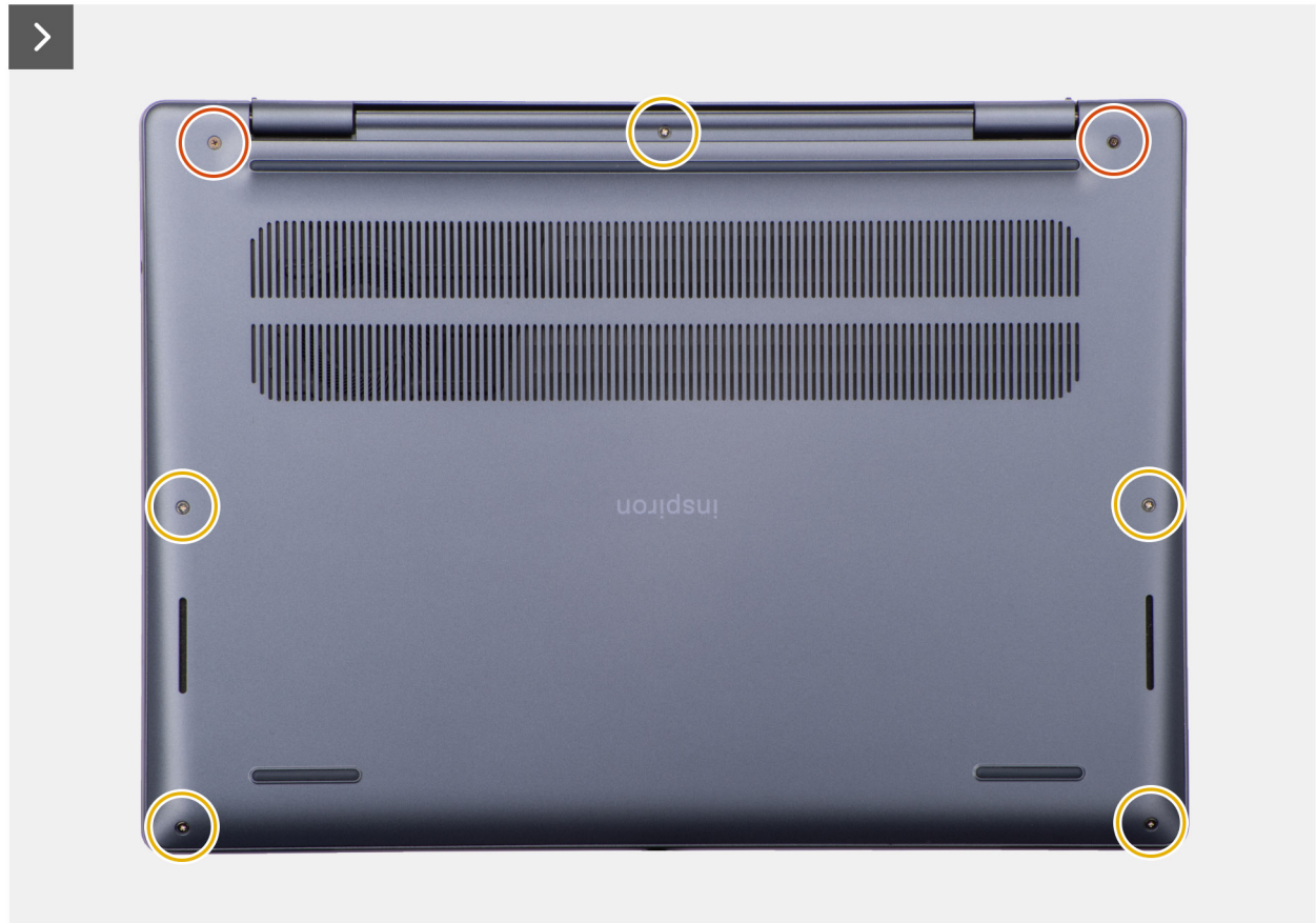
Figure 17. Removing the base cover
