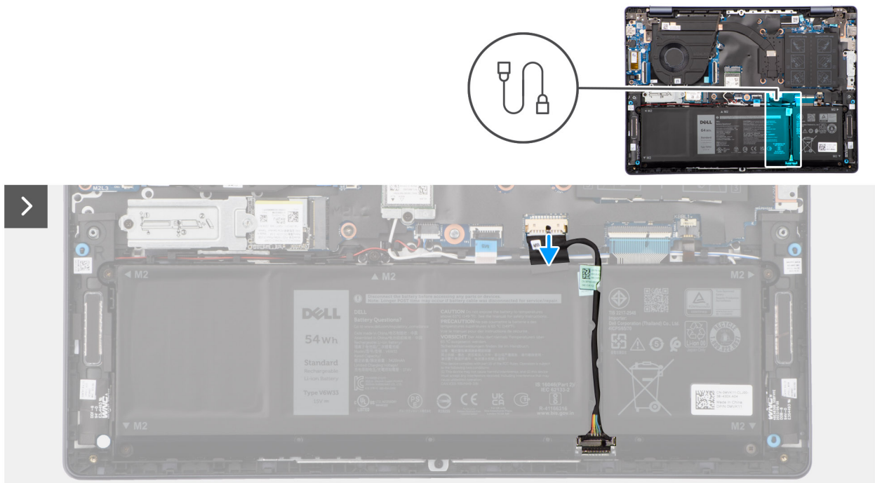
Figure 19. Disconnecting the battery cable
