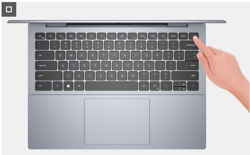
Figure 13. Pressing the power button to drain flea power
