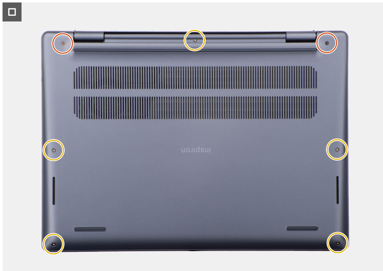
Figure 23. Installing the base cover
