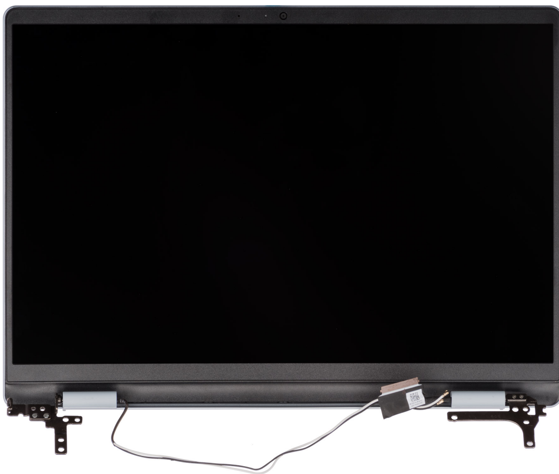
Figure 64. Display assembly (for computers shipped with a plastic chassis)
