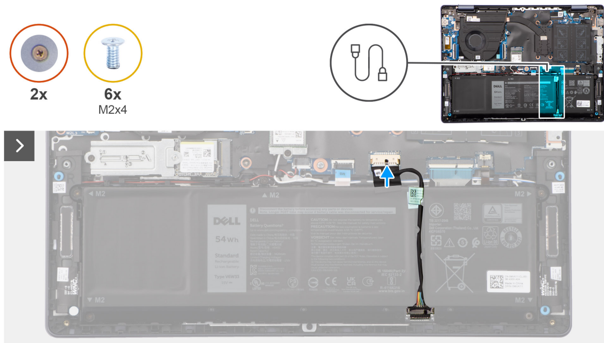
Figure 14. Connecting the battery cable
