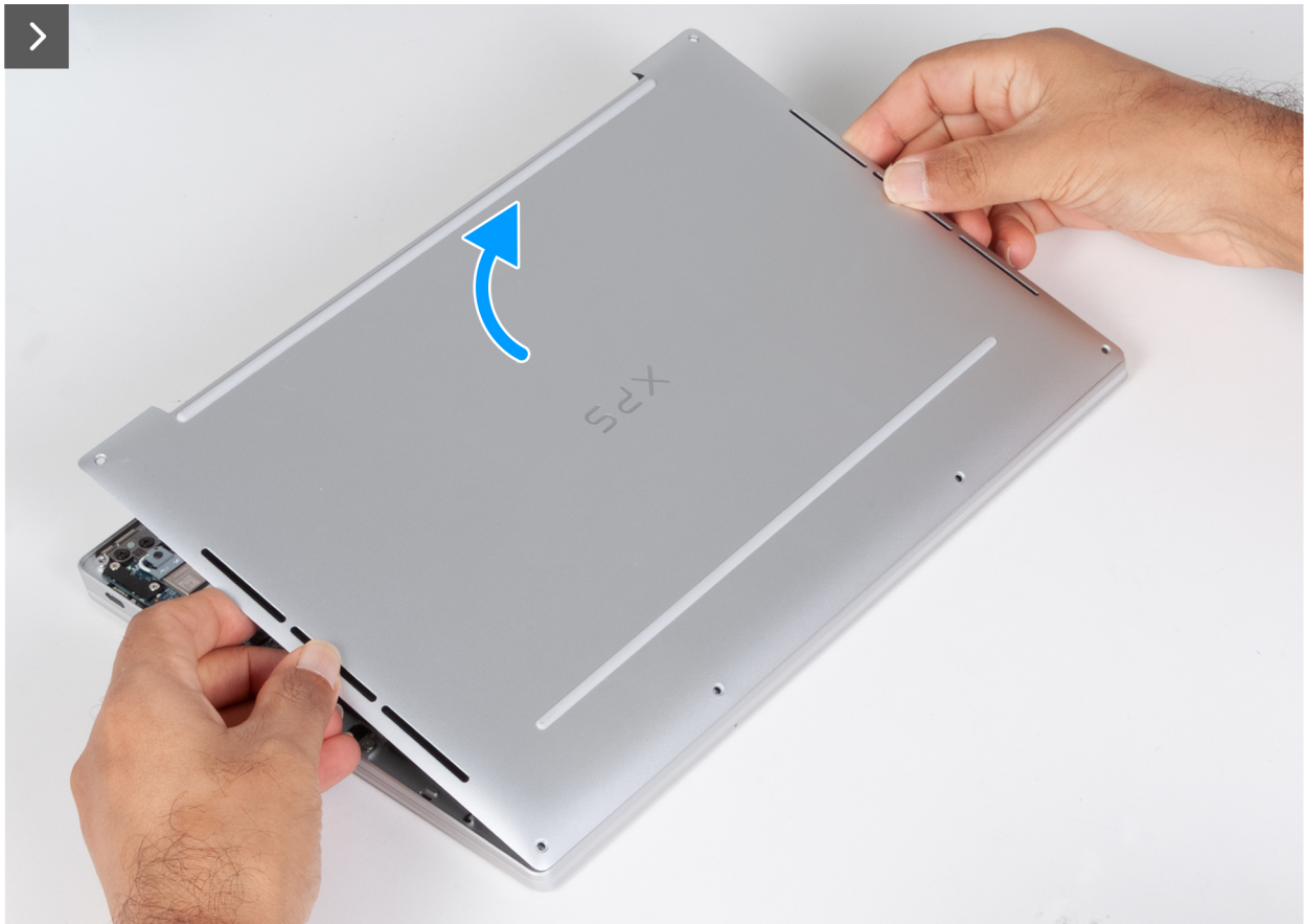
Figure 12. Removing the base cover
