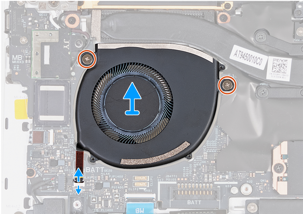
Figure 37. Removing the right/video fan
