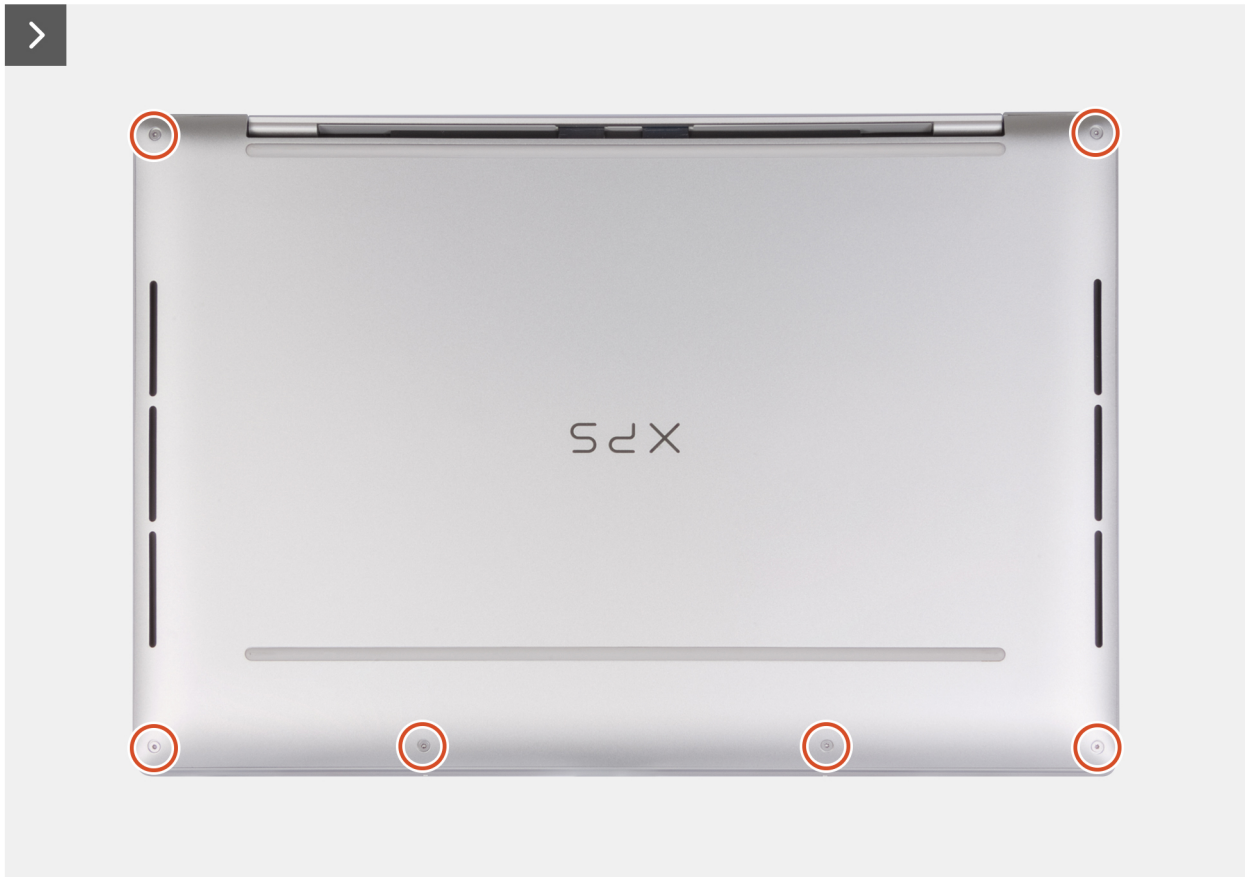
Figure 10. Removing the base cover
