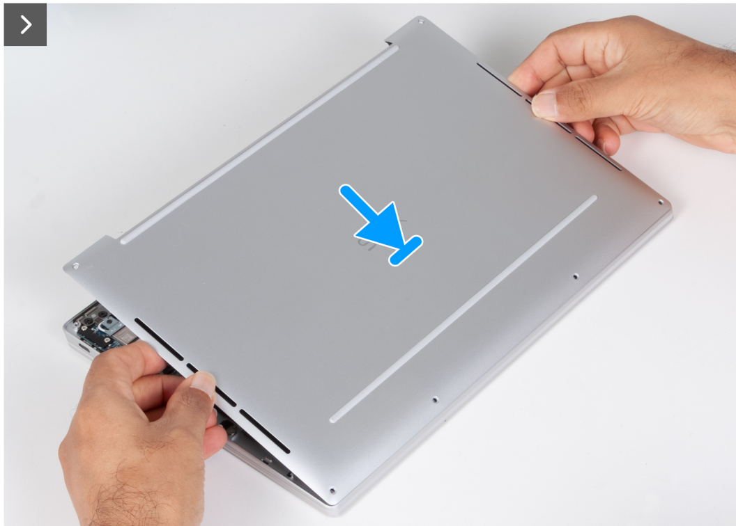
Figure 15. Installing the base cover
