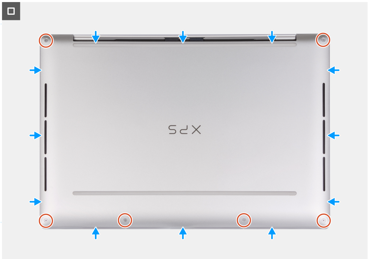
Figure 16. Installing the base cover
