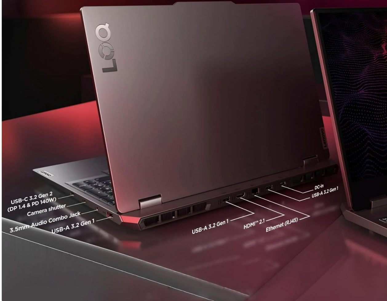
Figure 2.4: Side view of the laptop illustrating the available ports for connectivity, including HDMI output.
