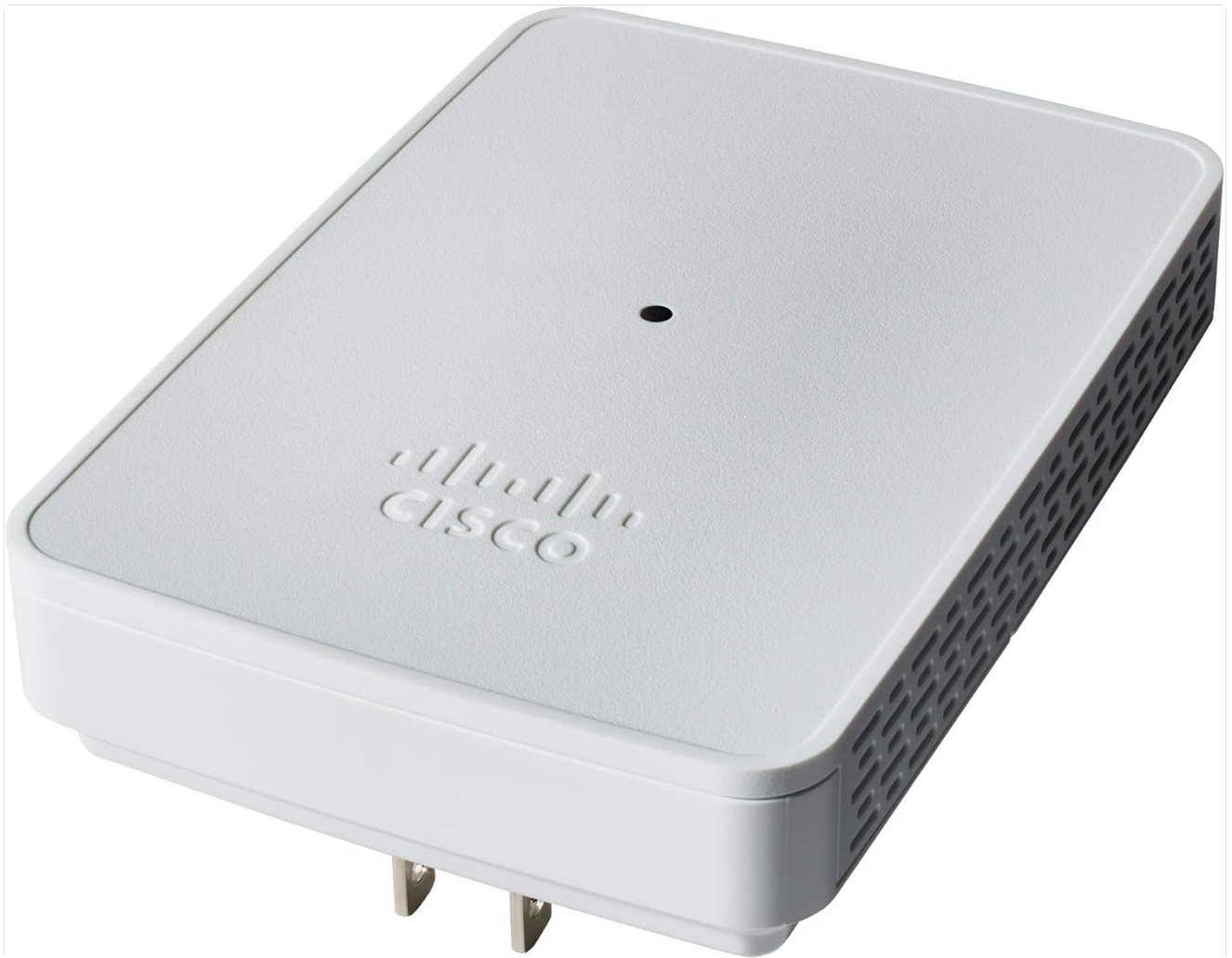
Image 1.1: The Cisco Business 142ACM Wi-Fi Mesh Extender. This device extends your wireless network coverage by plugging directly into a standard AC wall outlet.
