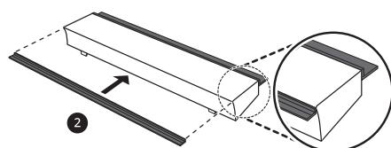
7 Attach the lower cover with the strip onto the appliance.
