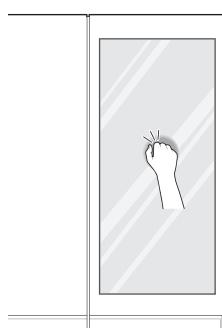
**1** Knock twice on the glass to turn the LED light inside the **Door in Door** on or off.
