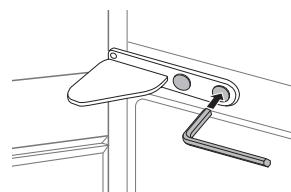
**2** Twist the hinge to raise the pivoting end so that the door can be lifted off. Lift the door off the lower hinge pin and remove it.
