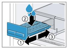
**Note:** If it is filled with too much drinking water, this may impair the function of the ice cube maker. The ice cubes cannot be removed individually from the ice cube tray. Too much drinking water was added and is running into the ice cube container, causing any ice cubes to freeze together.
