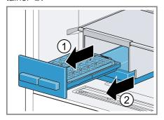
2. Lift the fixed shelf with the holder at the rear 1) and remove it 2).
