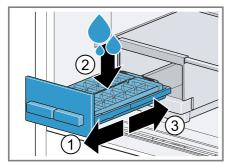
Note: If it is filled with too much drinking water, this may impair the function of the ice cube maker. The ice cubes cannot be removed individually from the ice cube tray. Too much drinking water was added and is running into the ice cube container, causing any ice cubes to freeze together.
