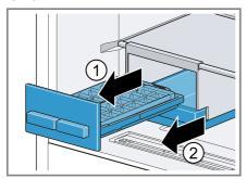
2. Lift the fixed shelf with the holder at the rear ① and remove it ②.
