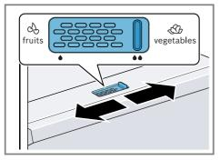
The air humidity in the fruit and vegetable container can be set according to the type and amount of food to be stored by moving the humidity control:
