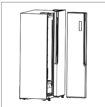
4. Lift The Door and Place it on a Soft Pad. Then Remove Another Door as Same Process.
