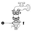
4 Check for water leakage.
