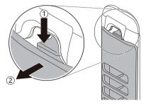
the filter into the wash drum. Press the top of the filter until you hear a click sound.
