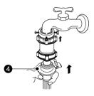
4 Check for water leakage.
