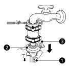
2 Take off the water filter from the tap by turning it clockwise
