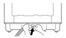
2 To change the direction of the drain hose, remove it and reinstall it facing in the correct direction.
