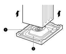
**2** Remove the foam tub insert.
