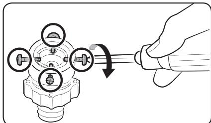
2. Use a Philips screwdriver to loosen four screws on the adaptor.
