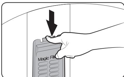
1. Press down the upper area of the filter case to remove.
