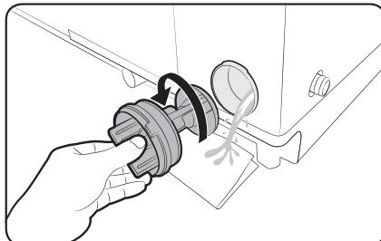
1. Put a floor-cloth or towel under the Pump filter. Turn the filter knob anticlockwise to remove.
