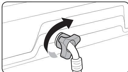
7. Connect the other end of the water hose to the inlet valve on the back of the washing machine. Turn the hose clockwise to tighten.
