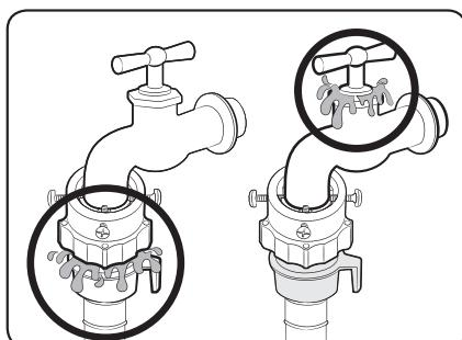
8. Open the water tap and check if there are any leaks around the connection areas.
