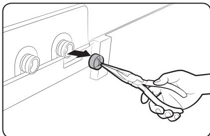
1. Use pliers to pull out the mesh filter from inside the water inlet as shown.
