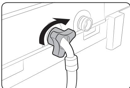
3. Reinsert the filter. Make sure it is tightened against water leaks.
