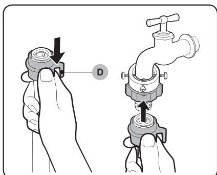
6. While holding down **part (D)**, connect the water hose to the adaptor. Then, release **part (D)**. The hose fits into the adaptor with a clicking sound.
