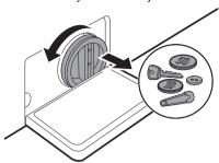
5 After cleaning the drain pump filter, carefully reinsert the filter and screw the drain cap back in clockwise carefully to avoid cross threading and leakage. Reinsert the plug back into the drain tube and place the tube into its holder.
