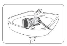
Clean the drain filter using a soft brush. While the drain filter is removed, make sure the impeller inside the drain pump is free of debris.
