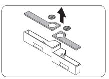
3. Remove the lids of both dispensers using the pull tabs at the back of each lid.
