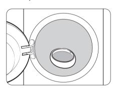
Pour the recommended amount of liquid or powdered detergent (specialty detergent) into the Aqua Pebble, and then put the Aqua Pebble directly into the drum. There are two guidelines inside the Aqua Pebble to indicate 50 ml (1.69 fl oz) and 100 ml (3.38 fl oz). Do not exceed the 100 ml line.
