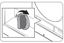
7. Reinsert the drain filter, and turn the filter knob to the right.
