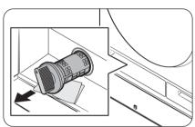
5. Turn the drain filter knob to the left, and drain off the remaining water.
