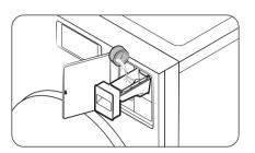
Apply additives such as fabric softener. Do not exceed the  $\max$  line.
