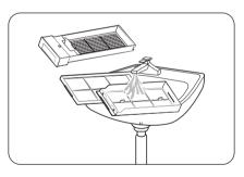
**4.** Remove lint on both inner and outer filters. Then, wash the filters in running water and completely dry the filters in a shade.
