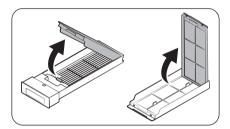
**3.** Open the outer filter, and then remove the inner filter.
