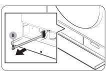
Put an empty, spacious container around the cover, and stretch the emergency drain tube to the container while holding the tube cap (B).
