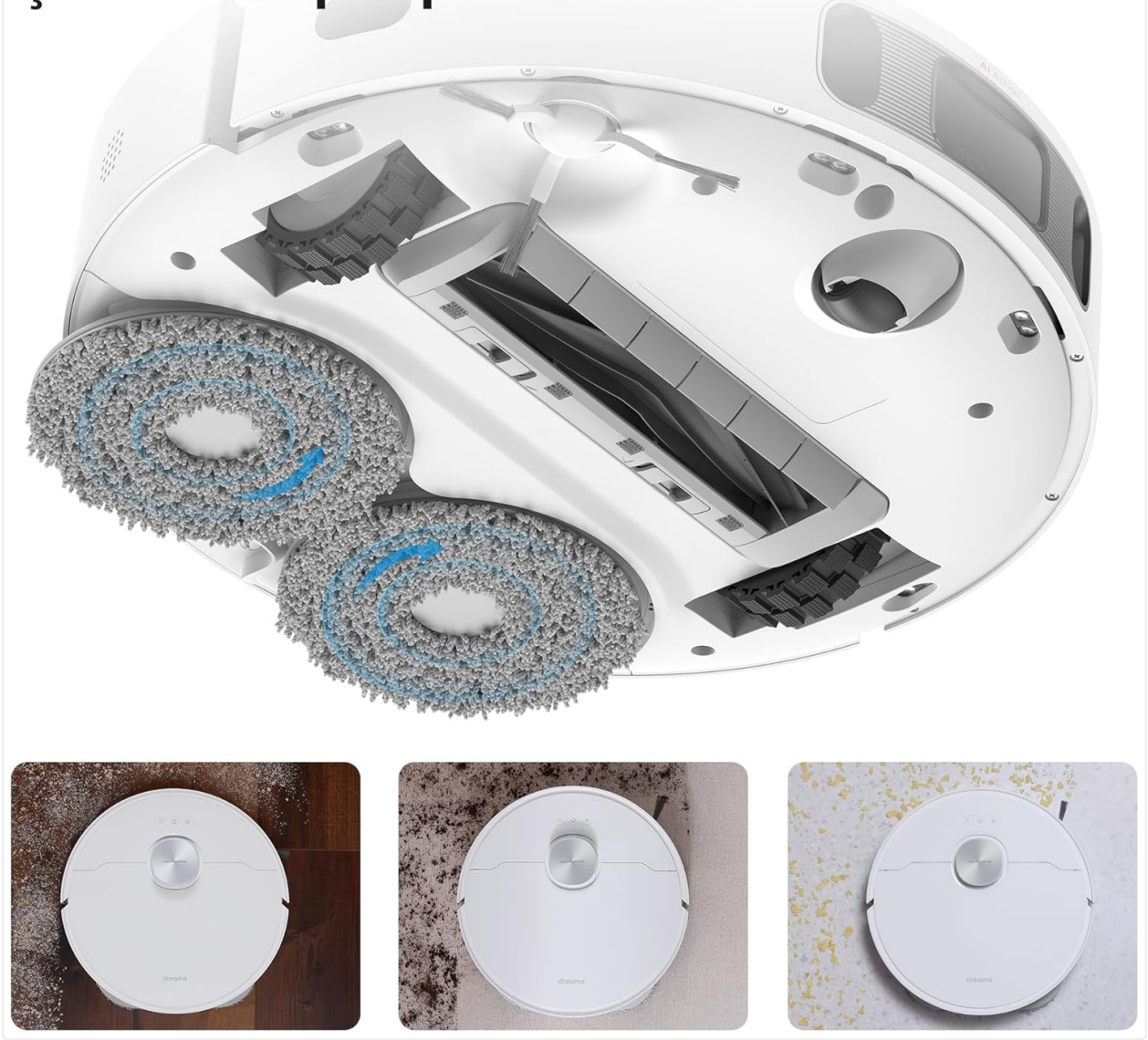
Figure 4.2: Automatic Dust Emptying and Mop Cleaning System
